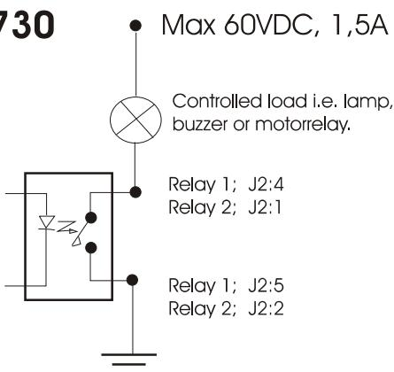
**U2384 Universal output board with 4 semiconductor DC relays.**
